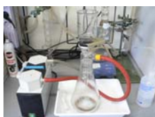
Figure 3: a) Apparatus for the preparation of the self-supported SWCNT anode with vacuum pump
