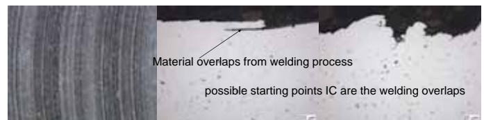
Fig. 2: Representative examples of Scanning Kelvin Probe Force Microscopy (SKPFM) and optical microscopy (surface and cross sectional) images after ASTM G110-92 for the clarification of intergranular corrosion of the Al/Al-5754 weldment. The specimen Al/Al-5754 show no intergranular corrosion whatsoever. Nevertheless, there is a kind of pitting corrosion that takes place on the samples that is dependent on the alloy composition. The results obtained by SKPFM on a FSW Al/Al-5754 weldment depict the dependency of the Volta potential differences on the particle number and size of the intermetallic phases.
