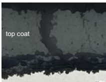
Fig. 3 YSZ Top Coat Failure
