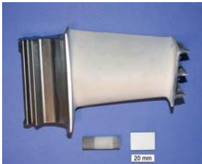
Fig. 1 A real TBC coated turbine blade and smaller laboratory oxidation sample.
