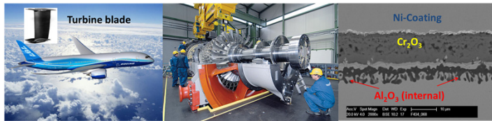
Fig. 1: The turbine blades for aircraft engines and gas fired power stations are manufactured with an Al-rich bond coat and a TBC.
