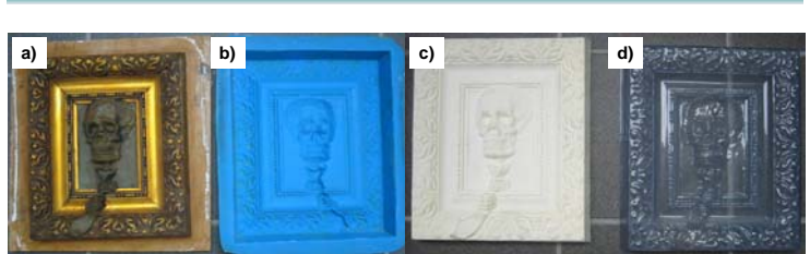
Figure 8: Image sequence to illustrate the production process of a thermoforming mould and the final formed plastic. An art object was used to serve as illustration object with high amount of detail and fine structures to be reproduced (a). A silicon negative form is produced from the art object (b). Filling the silicon form with slurry ceramic of optimized layer composition results in the thermoforming mould (c). The mould has shown very good performance in first vacuum forming tests as can be seen from the resulting plastic (d). In contrast to many state-of-the-art materials used for thermoforming moulds no water cooling of the mould was necessary during the plastic forming process.
