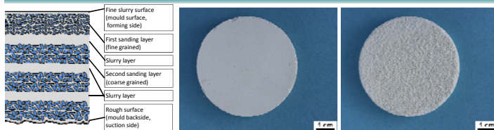
Figure 1: Schematics of a layered slurry ceramic (left) and photographs of surface (center) and backside (right) of a slurry derived ceramic plate.
