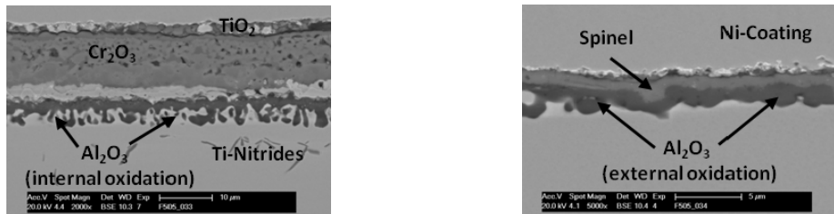
Fig 1: Left micrograph: Untreated IN738 after oxidation (24h/1050°C/air). Right micrograph: F-Implanted sample of IN738 ( 10^{17} F cm -2 / 38 keV) after oxidation (60h/1050°C/air).
