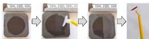
Fig. 3: Sequence of images illustrating the mechanical biofilm harvest from an anode.
