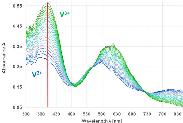
UV/VIS measurement via bypass through 0.1 mm flow-through-cuvette during charging the negative half cell (interval: 10 minutes)
