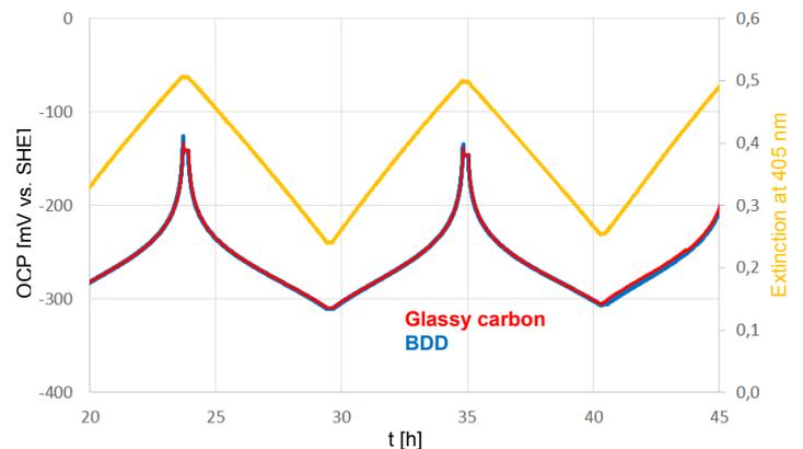
Extinction of the negative electrolyte at 405 nm and OCP of the negative electrolyte measured at a glassy carbon- or a BDD- rod during charging- and discharging
