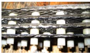
Fig.1: Stack of 4 pairs of BDD electrodes with Nafion® membranes as Solid Polymer Electrolyte (SPE). Scaling can be observed between BDD and membrane.
