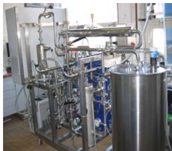
Fig.2: Technical loop for testing BDD stacks with different polarisation routines.
