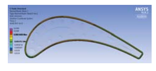
Calculated temperature distribution and resulting cooling strain in TBC
