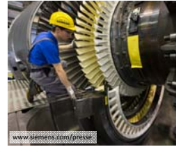
Fig. 2: TBC coated blades and vanes inside gas turbine.
