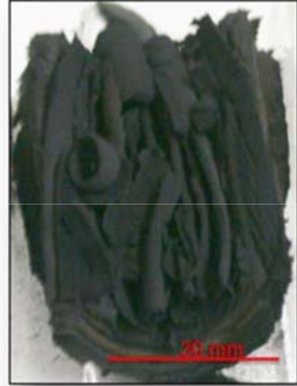
uncoated low alloy steel (1%Cr; 0.4%Mo) after 100 h under metal dusting conditions at 650°C (H 2 -24%CO-2%H 2 O)
