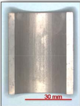
Ni Sn coated low alloy steel (1%Cr; 0.4%Mo) after 100h under metal dusting conditions at 650°C (H 2 -24%CO-2%H 2 O)
