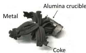
Metal sample attacked by metal dusting
