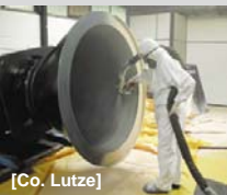
Figure 2: Photo of slurry application on a compound
