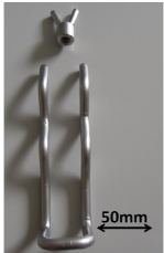
Fig.1: Anchors for refractory linings
