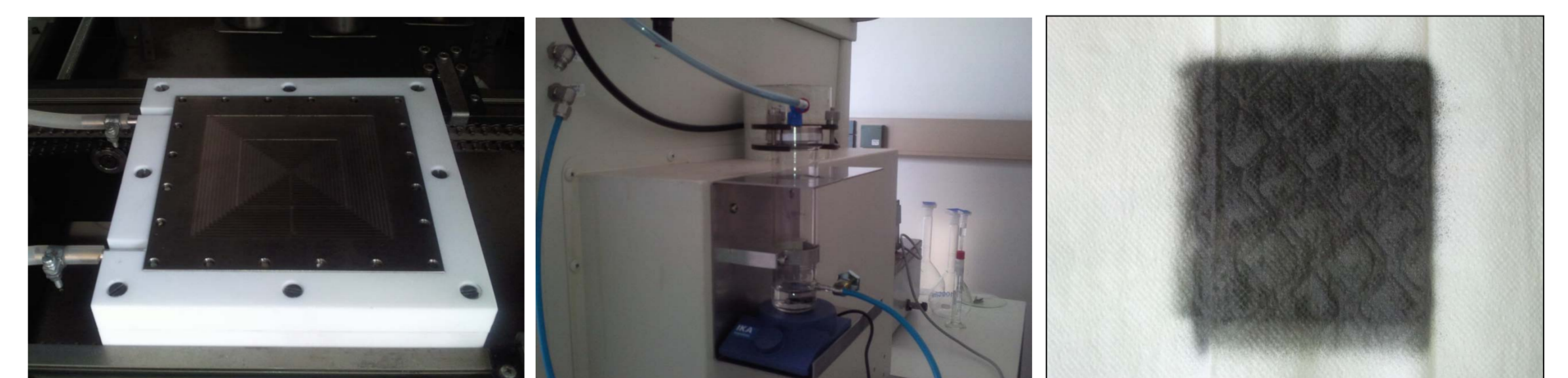
Fig. 3: Heating plate (left), ink reservoir (middle) and two carbon layers on a paper substrate (right)
