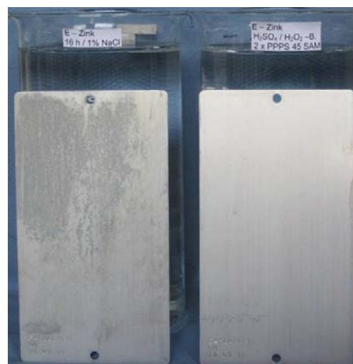
Fig. 3 : Electrogalvanised steel sheets (10.5 cm x 19 cm) after 16 h dipping in aerated 1% NaCl. Left : electrogalvanised steel only degreased by a mild alkaline treatment. Right : Analog galvanised steel sheet, but with additional acid pretreatment and coating with PPPA – SAM.
