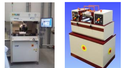
Fig. 2: (Left) Spray coating machine and (right) calender
