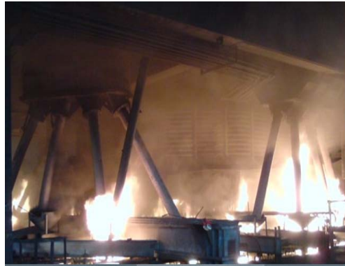
Fig. 34: Spark Ignitions on the power supply of electric arc furnaces in the Nickel production process (LARCO)
