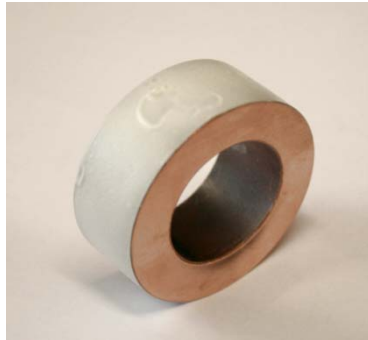
Fig. 37: Copper cylinder coated by electrical insulation layer sintered at 200°C
