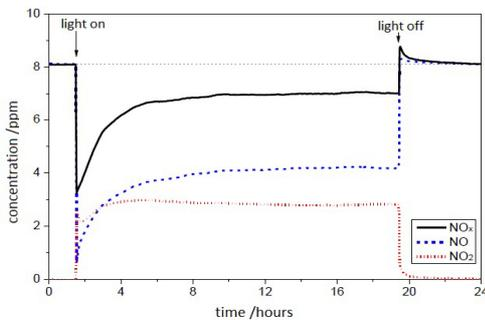
If the NO<sub>2</sub> concentration is measured during a photocatalytic NO oxidation test, it becomes clear that the release of NO<sub>2</sub> is a critical problem. In most cases, only about 30% of the introduced NO is transformed into nitrate. The rest is just oxidized to NO<sub>2</sub>.<sup>[3]</sup> It is also produced by the catalyst in the case of surface saturation with nitrate. Additionally, the behavior of ozone in combination with photocatalysts is still unclear.
