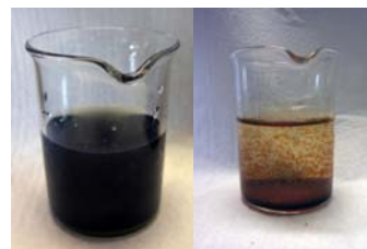
Fig. 4 : SDS-EG-MEEA-nZVI after aeration. The left image shows the sample 4 hours after aeration and the right image shows the sample after 18 hours aeration
