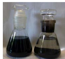
Fig. 3 : SDS-EG-MEEA-nZVI (left) and EG-MEEA-nZVI (right) 30 minutes after addition of drinking water Both samples were stored under nitrogen atmosphere
