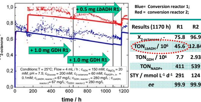
The synthesis runs very stable over a period of more than 1200 h. Turnover numbers ( $\text{mol}_{\text{product}}/\text{mol}_{\text{catalyst}}$ ) for both enzymes are extremely high.
