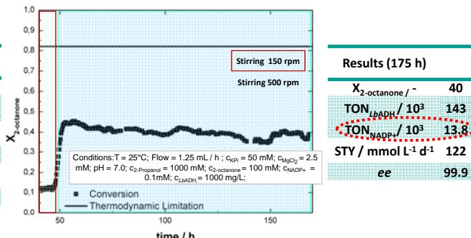
The synthesis runs stable over a period of more than 170 h. The turnover numbers ( $\text{mol}_{\text{product}}/\text{mol}_{\text{catalyst}}$ ) for the cofactor NADP<sup>+</sup> is very high.
