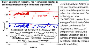
the inlet concentration also leads to a stable process and halves the cofactor cost. Due to the higher ratio LbADH/GDH in reactor 2. an average of 0.025 mM of the cofactor can be used for recycling at a TON<sub>NADP+</sub> of 940 per cycle. In total, the cofactor utilisation can be increased ~4fold as revealed by cofactor stability tests and 500kinetic modelling.
