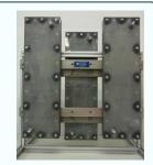
Pilot plant for adsorption and desorption: 3 separate cells, 50 x 15cm<sup>2</sup>, 360mL GAC/chamber
