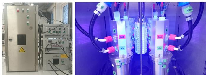
Four equal reactors with a volume of 25 ml are arranged around a 20 W (light flux) lamp with 365 nm LEDs. The temperature of the reaction media and the light intensity can directly adjusted. The reactors are equipped by gas connections to work under oxygen free conditions. The hole set-up is installed in fully closed "photocabinet" to protect the environment from the UV-light.
