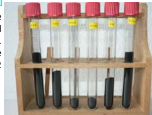
Fig.2: Volume evaluation of 1g of each carbon in Ø11,3 cm tubes.
